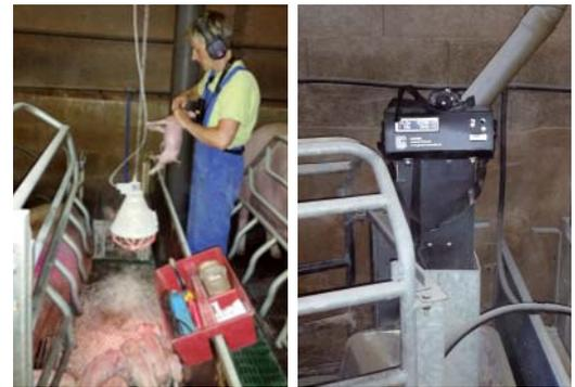
Photo 1: on the left: personal air sampler during the teeth clipping – on the right: dust measurements with Grimm spectrometer
